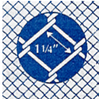
Figure 8: Chain link fence with 1.25" mesh to discourage climbing by young children
